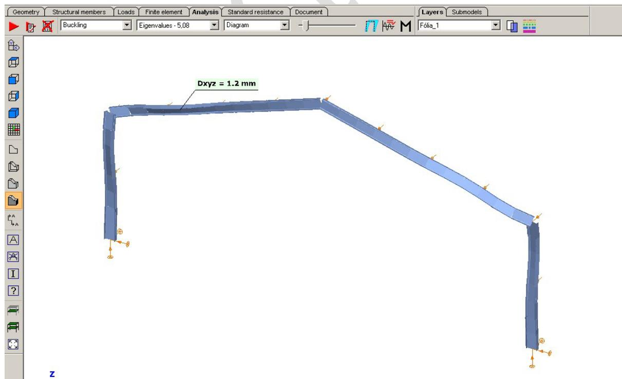
The first eigenvalue which indicates lateral torsional buckling mode is the following (EN 1993-1-1 6.3.4 (3)):
