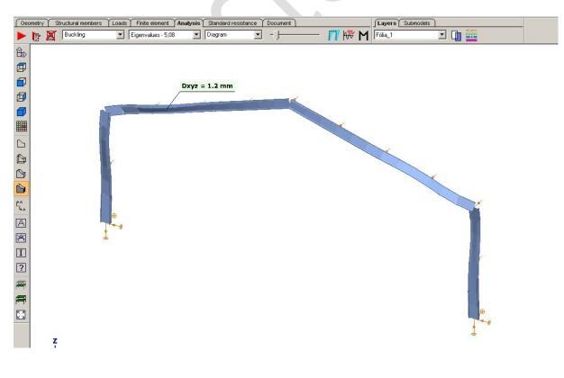
The first eigenvalue which indicates lateral torsional buckling mode is the following (EN 1993-1-1 6.3.4 (3)):
