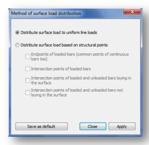
Converting the surface load to line loads based on structural points has the following background:
