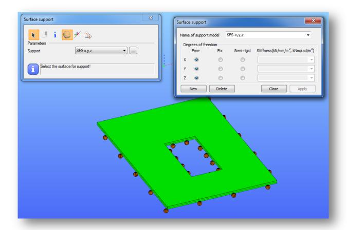
By clicking on a plate object, all the surface of this selected object will be supported by the support.
