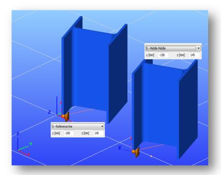
If the eccentricity of the columns is changed to y= 100mm, the new position of the supports is as follows:
