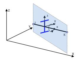
In case of a generally positioned beam member (not column with vertical reference line) the plane defined by the local "xz" system takes always vertical position and the axis "z" points towards the positive "Z" direction. For beams with (single) curvature the axis "x" is always the tangent.
