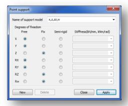
The support type names can be clearly understood. For instance "x,y,z, xx" means any movement is fixed in x, y and z direction and the rotation around x axe is also fixed. All the rest DOFs are free.
