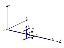
In the basic case the local coordinate system of a bar can be determined considering its reference line ("x") identical to the global axis "X". In this case the direction of local axes "y" and "z" are identical to the global axes "Y" and "Z". The position of the cross section on the bar is the following: the reference line goes through its centre of gravity, and the section "YZ" system coincides with the local "yz" system of the bar.
