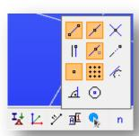
Snapping the end points of graphical (lines, arcs) and structural (beams, columns) objects
