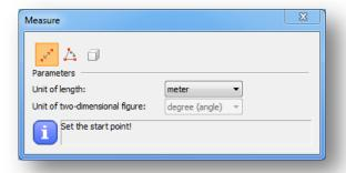
Measure distance: Shows on the screen the measured distance between two picked points in meter or in millimeter, selected from the "unit of length" list box.
