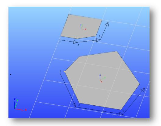
In case of surface elements the local coordinate system can be modified using the tools presented in Chapter 4.2.1.
