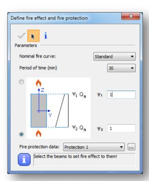
Different fire protection can be created by clicking on the three dot icon next the Fire protection data. In this window it is possible to select between Unprotected and Protected.
