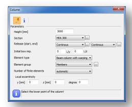
► Section: before creating a beam or column member cross-sections should be loaded, and the appropriate section can be selected from the combo including the loaded sections. If no section has been loaded in advance the Section dialogue can be called by pressing the button next to the combo. For more information about section administration see Chapter 9.2.
