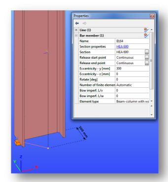
If the column is rotated with 45 degree, then the support moves together with the column.
