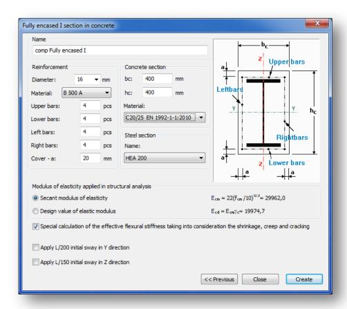
If the initial sways in the y and z directions were applied on the checked cross-section then the stability check of the composite columns can be neglected. Cross-section checks are enough.
