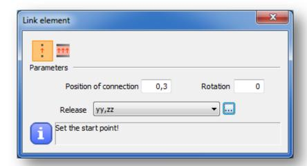
For example if there is a cantilever on a relatively high tapered column (see image below) it is advisable to connect it not directly to the reference line of the column but with the link element. If it is connected the way like that the analysis and design results are more accurate and the modelling is more exact.
