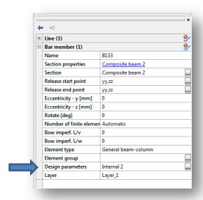
In the design parameters window you can set the distance between parallel beams, the number of shear studs, the type of analysis, moment redistribution and the support point positions along the member. The support position table can be automatically filled up by
