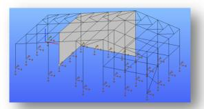
• wireframe view : on the wireframe view the lines of the cross sections and plate thickness appear, the supports are line types.
