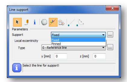
There are two default types for line supports the Fixed and the Pinned. With the <u>...</u> button it is also possible to define a new line support by giving the attributes of constrains as it is needed.
