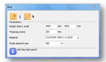
In the **PLATE** and **WALL** definition panels the drawing functions are collected in order to create the plate with the desired shape. Arbitrarily shaped holes can be defined in existing plate members. Three parameters can be set: the thickness, the material and the finite element size of the surface member. The finite element size is an approximate target maximum size for the finite element mesh used for the calculation of surface members.
