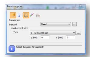
After selecting the coordinate system, the type of the support has to be selected from the list-box. There are several point supports types predefined.
