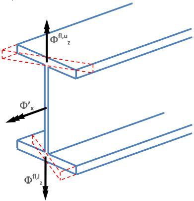
In this case the warping DOF can be considered as a dual and opposite rotation of the flanges about the axis perpendicular to their width (in this case the local axis "z").
