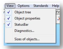
With the first four functions the visibility of the dockable windows can be switched. With the **SIZES OF OBJECTS...** function, the size of the objects can be changed.
