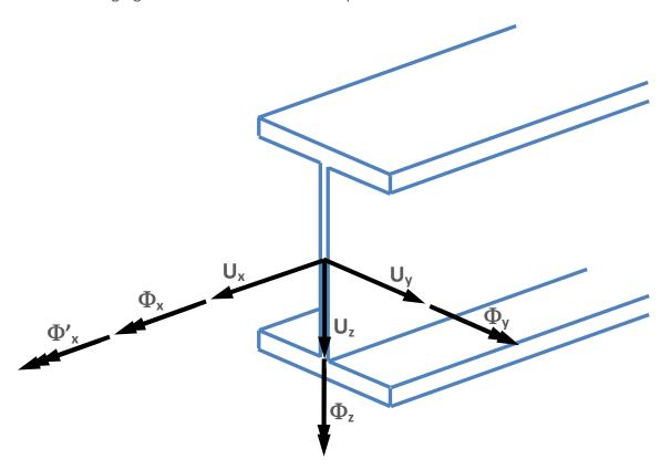
The first 6 DOF are the conventional displacements ( $U_x$ ,  $U_y$ ,  $U_z$ ) and rotations ( $\Phi_x$ ,  $\Phi_y$ ,  $\Phi_z$ ) according to the local coordinate system of the member (see section **4.2 COORDINATE**
