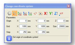
The User coordinates system can be switched on (or switch back to the global system) at the bottom status bar
