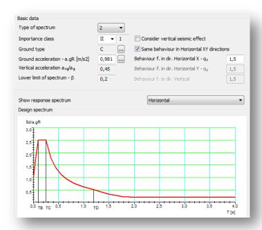
The standard design response spectrum can be defined according to the EuroCode 8. The parameters of the spectrum are automatically loaded from the selected national annex.
