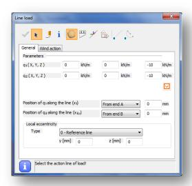
In order to place a line load click on the member using the select function ( ). Line load can be applied to multiple members at the same time by using **PLACE LOADS** icon ( ).
