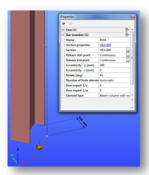
3. Example: The support is placed according to the global coordinate system, the eccentricity is 300mm in the z direction of the local coordinate system of the supported column relative to the middle-middle point of the section geometry.
