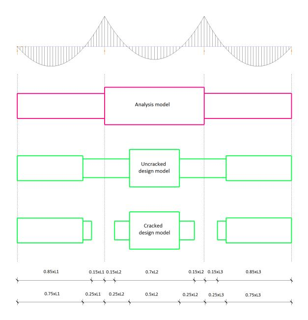
FIGURE: EFFECTIVE WIDTH IN ANALYSIS AND DESIGN MODELS
