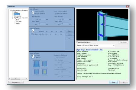
If the **BEAM** is selected in the connection tree, then beam related properties of the connection can be set like the section size and material grade (#1). Beam end configuration can be set such as haunch (#2). Furthermore the beam span and position of the beam are essential for the joint calculation (#3).
