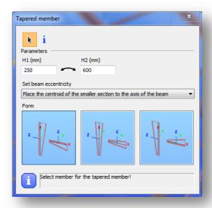
First the user has to specify the parameters and beam eccentricity options for the member to be tapered on the *TAPERED MEMBER* dialogue.
