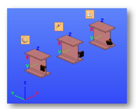
By changing the eccentricity of the supported object, the support will keep the orientation to the coordinate system which was used by placing the support.
