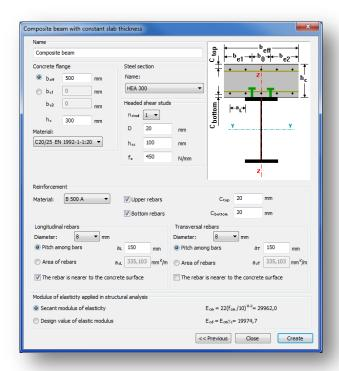
After the composite cross-section is defined it can be used for member creation the same way as a steel cross-section.
