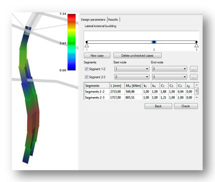
By clicking on the three dots icon the design parameters can be altered. The elastic critical bending moment can be calculated from the analytic formula or from the critical load multiplier. When the first method is used the factors can be typed in or a special automatic C factor calculator can be used by clicking on the AutoC button. The second option is to choose the corresponding critical load multiplier from the list.
