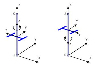
In case of vertical reference line (column members) the local axis "y" has the same direction as the global axis "Y", the direction of the local axis "z" depends on the placement of the column (position of the start and end points).
