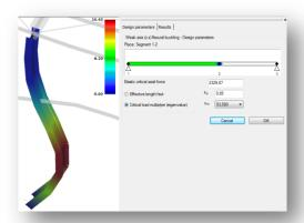
The actual segment is highlighted with green. There are two options to set the design parameters: set the effective length factor manually by typing in the appropriate value or by choosing the right critical load multiplier. The second option is possible if the special analysis has already been run. In both cases the elastic critical axial force is automatically calculated.
