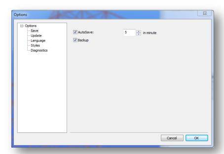
If **Autosave** is clicked, the program automatically performs a save periodically in accordance with the adjusted number of minutes. If **backup** is clicked, *ConSteel* creates a backup file *after manual save is performed*. The backup model file can be used as a normal model by removing the **.bak** extension.
