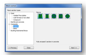
During the creation of the cross-section the parameters of the concrete section, reinforcement and the encased steel section have to be set.
