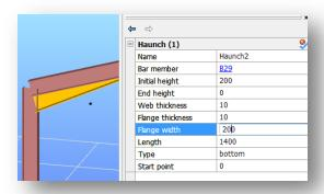
IMPORTANT TO KNOW THAT FOR THE HAUNCHED PART OF THE MEMBER NEW SECTIONS ARE CREATED DURING THE AUTOMATIC FINITE ELEMENT GENERATION WHICH CONSIST OF THE ORIGINAL SECTION AND THE HAUNCH WITH APPROPRIATE WEB HEIGHT. THESE NEW SECTIONS ARE PLACED ECCENTRICALLY ON THE REFERENCE LINE OF THE MEMBER (EXCEPT THE SYMMETRICAL HAUNCH TYPE).
