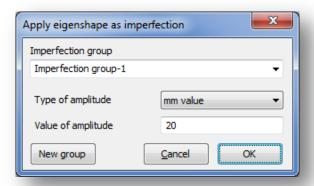
Pressing the  $\mathbf{OK}$  button the eigenshape is applied as an imperfection with the set parameters.
