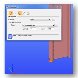
If the column is moved with 300mm in the y direction in the local coordinate system, then the position of the support will no change.
