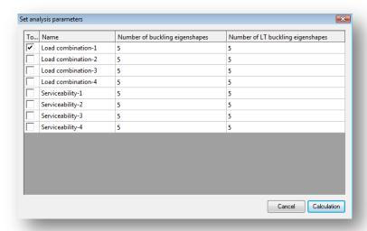
The next step is to choose the load combination and design type from the options: pure cases (strong axis buckling, weak axis buckling, lateral-torsional buckling) and interaction stability (interaction of buckling and lateral torsional buckling, interaction of buckling and bending, interaction of lateral-torsional buckling and bending). The dominant load combination is automatically selected and marked with a \* symbol.
