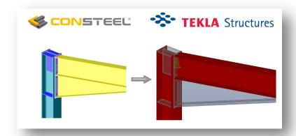
ConSteel uses Tekla Open API (Application Programming Interface), also known as the .NET API. This provides an interface for third party applications to interact with the model in Tekla Structures. Therefore both applications need to have installed in order to export model from ConSteel to Tekla Structures.
