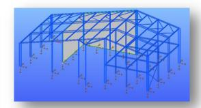
▶ hidden line view : the cross section and plate thickness appear in a solid form without shading and sparkling effects, the supports are solid types.
