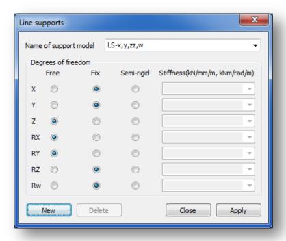
By positioning a line support the effect of the applied coordinate system and local eccentricity type are the same as for the point support.
