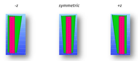
2. Place the centroid of the bigger section to the axis of the beam: the centre of bigger H value of the tapered member will be positioned to the axis of the original beam
