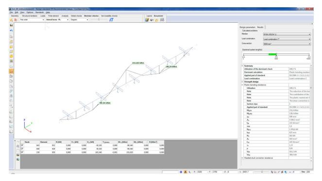
Effective width of the cross section and the optimal number and layout of the shear studs are automatically calculated during the analysis.
