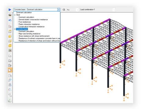
All of the possible standard checks can be performed such as bending, shear and torsion resistance for beams and interaction of compression and bending and shear resistance for columns. Furthermore, ConSteel checks the minimum and maximum EuroCode detailing rules.
