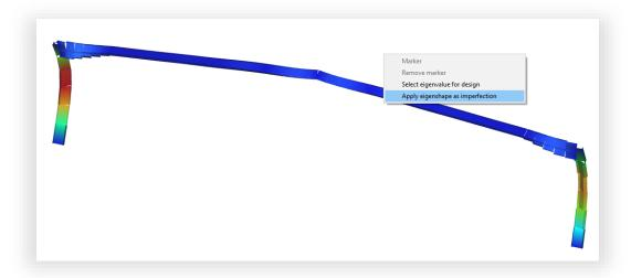
The new automatization, in case each load combinations, defines the proper direction of the imperfections and apply them accordingly during the analysis.
