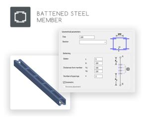
The macro can handle I, H or U section. Parameters of the battening plates, that can be placed symmetrically or unsymmetrically, can be set manually.
