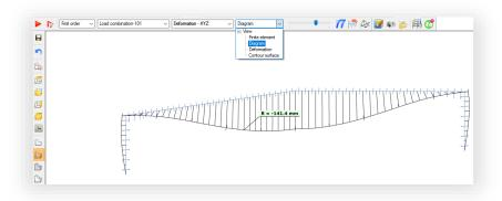
With the diagram view, not just the displacements can be visualized but the rotations and the warping results also. Result table was also extended with the warping results.
